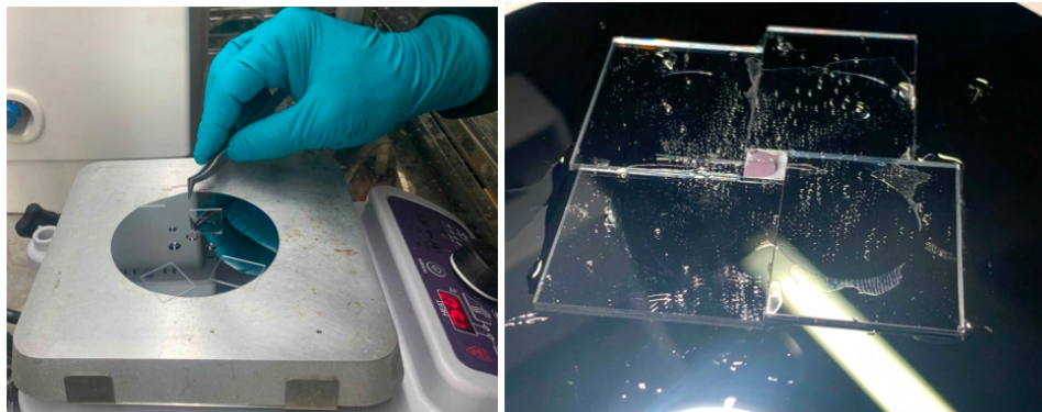
Figure A.7: Placing crystalline wax shards where sample and supports should be located (left) Image of mounted sample (right)
